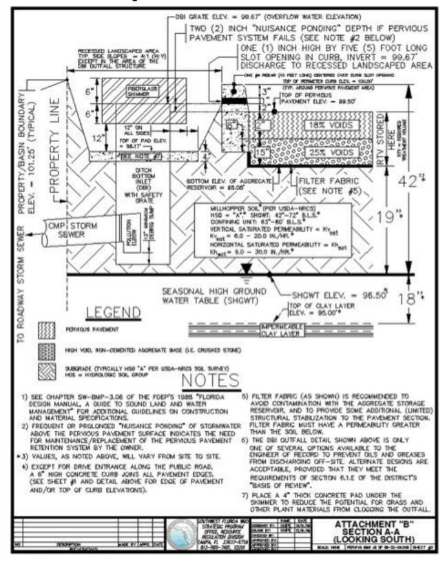
Figure 5.9.9. Pervious Pavement Site Plan
