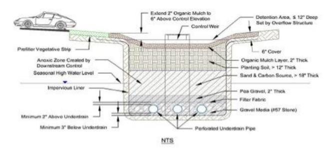
Figure 5.15.3. Example Cross Section View for Nitrate Removal with Overflow
