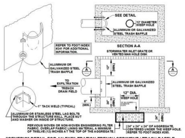
Figure 5.4.3. Detail for Exfiltration Trench Trash Baffle
