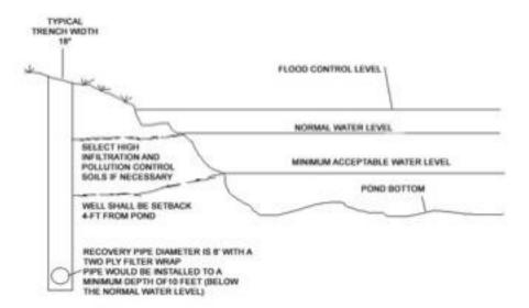
Figure 5.12.2. Schematic for a Typical Stormwater Harvesting Pond
