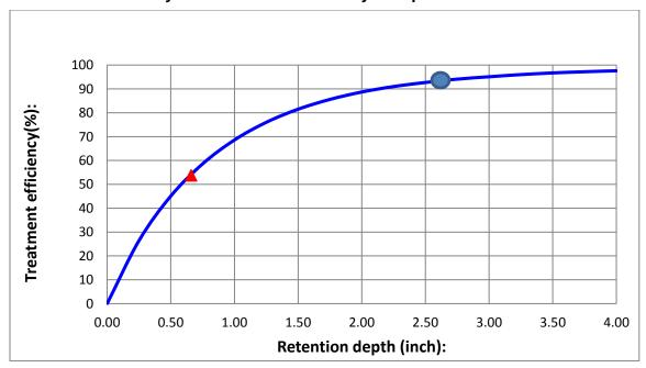
Figure 5.15.7. Example Average Annual Runoff Capture Efficiency of a Biofiltration System in Escambia County for Specific Conditions
