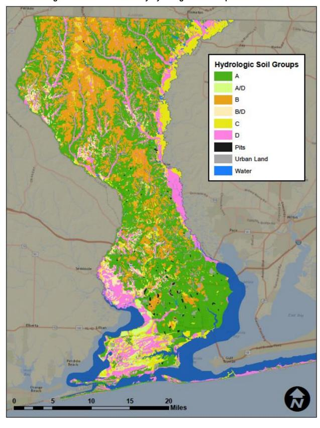
Figure 2.1. Escambia County Hydrologic Soil Groups Distribution
