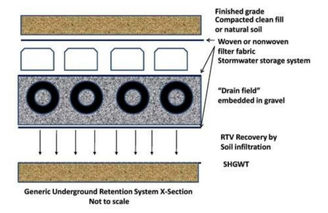
Figure 5.5.1. Generic Underground Retention System
