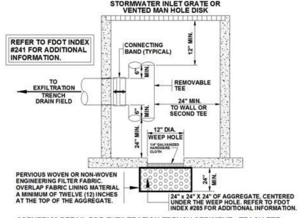
Figure 5.4.4. Generic Detail for a Typical Exfiltration Trench Trash Tee
