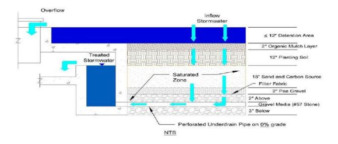
Figure 5.15.4. Example Stormwater Planter Box Biofiltration System
