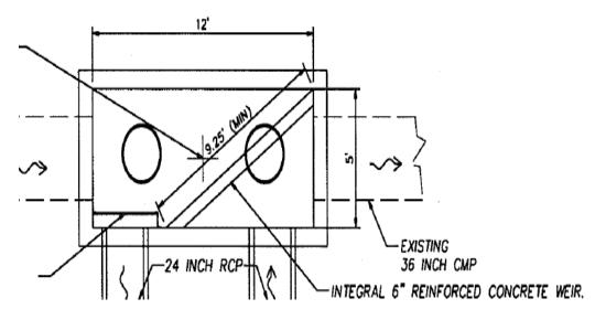
Figure 5.13.1b. Top View of Diversion Box to Off-Line Filter
