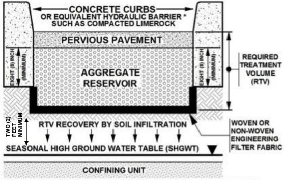
FIGURE 5.9.1. Typical Pervious Pavement Cross Section
