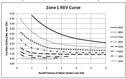
Figure 5.11.1. Rate Efficiency Volume (REV) Curve for a Rainwater Harvesting System in Escambia County with Constant Daily Demand
