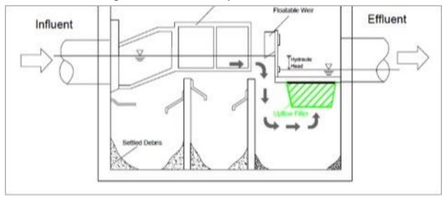
Figure 5.13.1a. Off-line Up-Flow Filter Schematic
