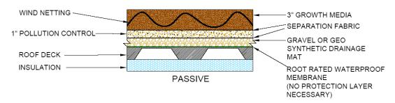
The root zone is comprised of the growth media and the pollution control media. A permeable fabric is used on both sides of the pollution control media to separate it from the soil or growth media layer above and a drainage layer below. A membrane, impervious to water and plant roots, is placed under the drainage layer to isolate the green roof system from the structural members of the building.
